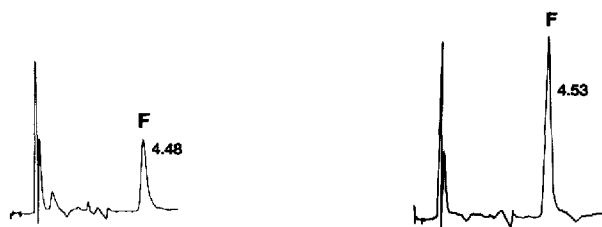
Fig. 3. Typical chromatogram from plasma obtained by analysis according to the described method. The sample, collected 8 h after intravenous administration of 45 mmol of foscarnet, contained 79 \mu\text{mol/l} foscarnet (F).
